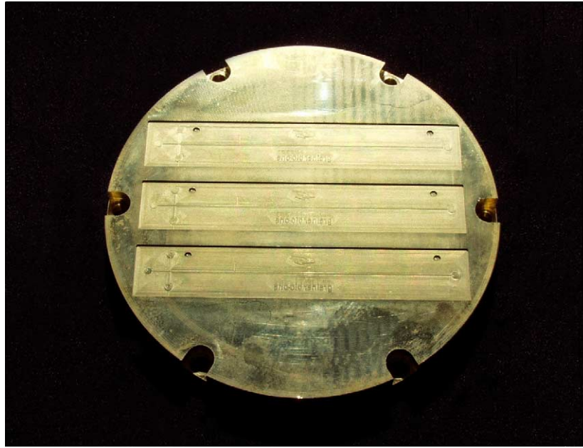
Fig. 3. General view of the metal mold insert made of brass with three identical fabrication areas.
