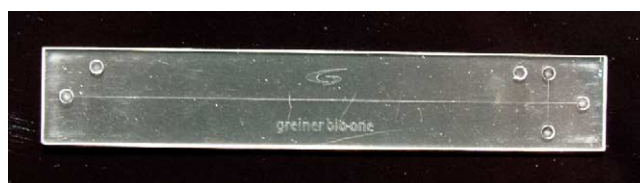
Fig. 7. Covered CE chip in the microscope slide format.
